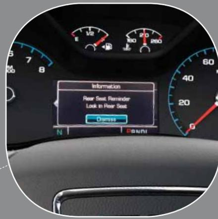
**Rear-Seat Reminder** This feature is activated when a second-row door is opened or closed during or just before a trip. When Canyon is turned off, under certain conditions, an audible chime and a message in the Driver Information Center remind you to check the second row.<sup>2</sup>
