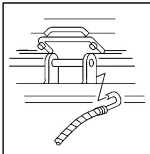
5. Hook the cable onto the outside portion of the liftgate hinges.
