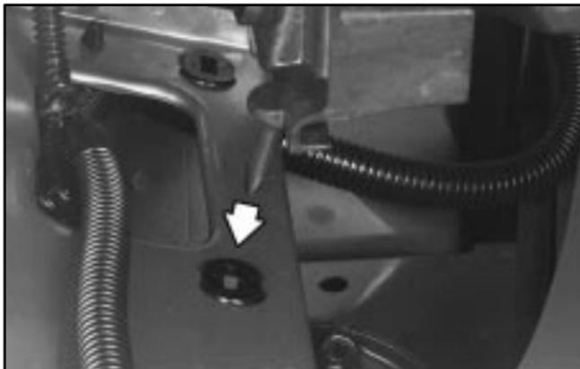
9. Align the pins on the bottom of the headlamp assembly with the holes in the lamp support bracket while placing the holes in the assembly over the bolts where the wing nuts attach.
