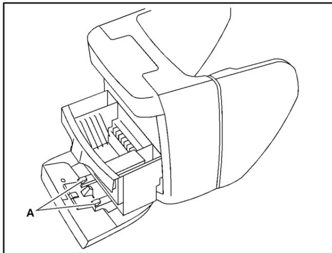
To remove the tray, slide it almost all the way out. Don't let the tray lock over the plastic tabs at the end of the guide rails (A). Lift the tray out of the guide rails. The rubber mat under the tray also lifts out for cleaning. When the rubber mat is put back in, be sure the tabs at the back of the mat are seated in the slots at the back of the storage bin.
