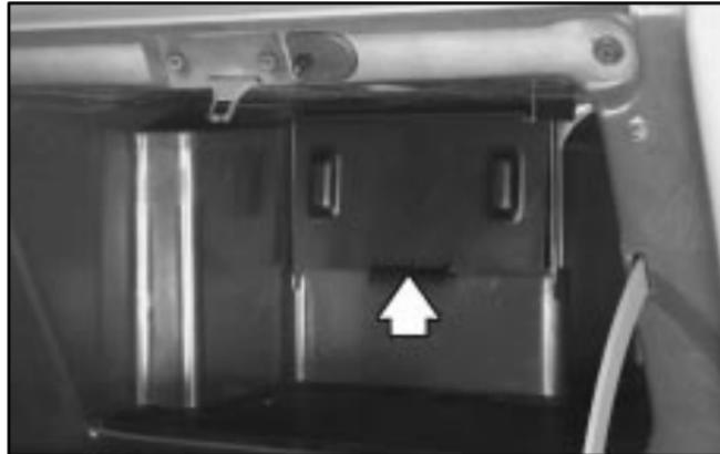
1. Pull the tab located on the outer access panel up and out.
