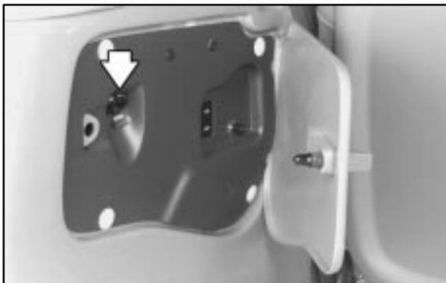
The rear accessory power outlet is located in the rear compartment on the driver's side next to the air inflator system.
