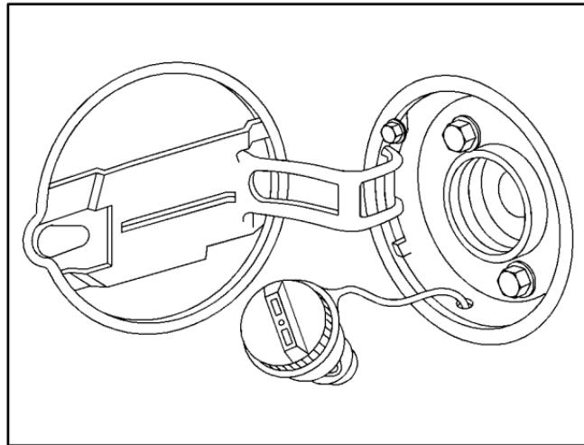
While refueling, let the cap hang by the tether as shown. To remove the fuel cap, turn it slowly to the left (counterclockwise). The fuel cap has a spring in it; if you let go of the cap too soon, it will spring back to the right.
