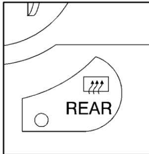
Press the REAR button to warm the defogger grid on the rear window and to turn on the heated outside rearview mirrors.
