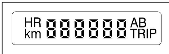
In addition to the standard odometer, the cluster can also display two separate trip odometers (designated by the letter A or B in the display window) as well as your vehicle's Engine Oil Life (designated by the word OIL in the display window). The display can be toggled between the odometer, the trip odometers and engine oil life by quickly pressing and releasing the trip/reset button located to the right of the temperature gage.
