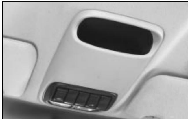
The front overhead console includes two reading lamps, a storage compartment and a switchbank.
