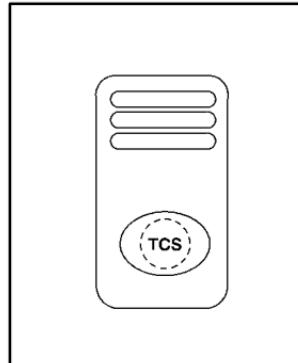
To turn the system off, press the TCS button on the instrument panel switchbank.
