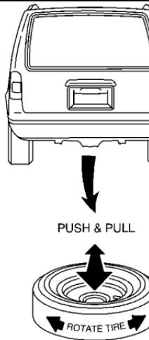
6. Make sure the tire is stored securely. Push, pull, and then try to rotate or turn the tire. If the tire moves, use the folding wrench to tighten the cable.
