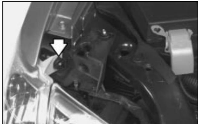
2. Remove the thumbscrew attaching the front turn signal/parking lamp assembly to the headlamp assembly.
