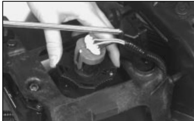
4. Unscrew the black retainer ring that holds the bulb assembly in place.
