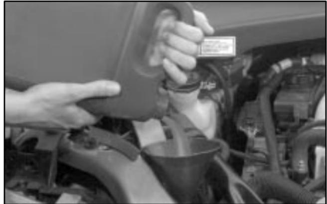
4. Fill the radiator with the proper DEX-COOL® coolant mixture, up to the base of the filler neck. See "Engine Coolant" in the Index for more information about the proper coolant mixture.
