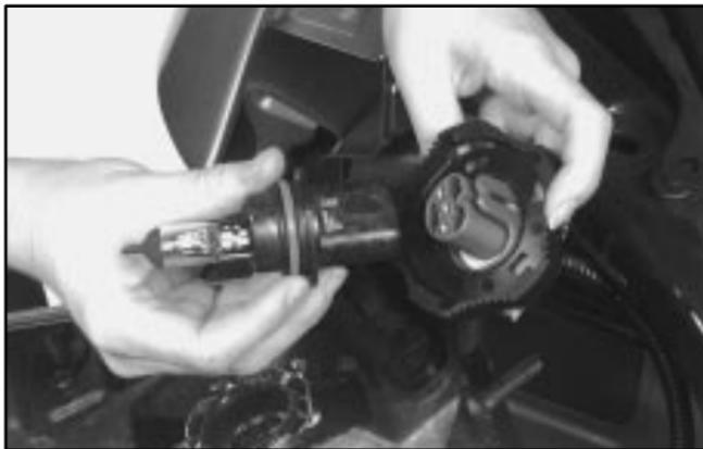
7. Install the new bulb through the black retainer ring and into the electrical connector. Tighten the black retainer ring in place. Push the bulb firmly enough so that the blue tabs hook over the tab on the bulb.
