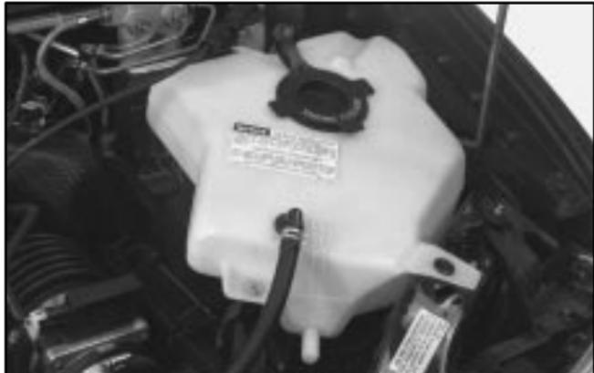
The engine coolant reservoir is located on the driver's side of the vehicle, above the engine air cleaner/filter. See "Engine Compartment Overview" in the Index for more information on location.
