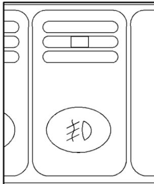
The fog lamps switch is located in the instrument panel switchbank. Press the fog lamp symbol on the switch to turn on the lamps.
