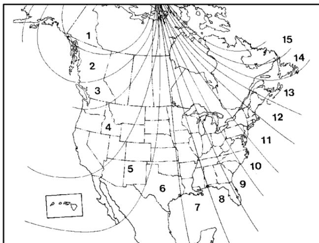
Turn the ignition on and cycle the DIC to the compass/temperature mode. Press both the E/M and MODE buttons simultaneously for approximately five seconds. The last entered variance zone number will be displayed. Press the E/M button until the proper variance number, as shown on the map, is showing. Press the MODE button to set the new variance zone and resume normal operation.
