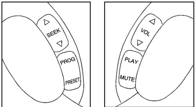
**SEEK:** Press the up arrow to tune to a higher radio station and the down arrow to tune to a lower radio station. The sound will mute while seeking. When playing a cassette tape or compact disc, press SEEK to hear the next selection.
