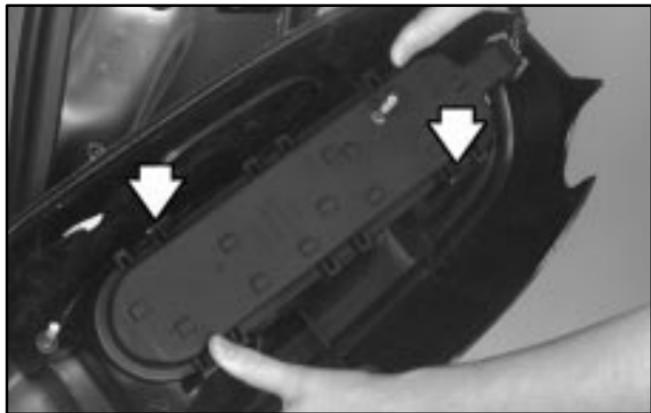
4. Remove the bulb holder by pressing the four retaining tabs and pulling the holder away from the assembly.
