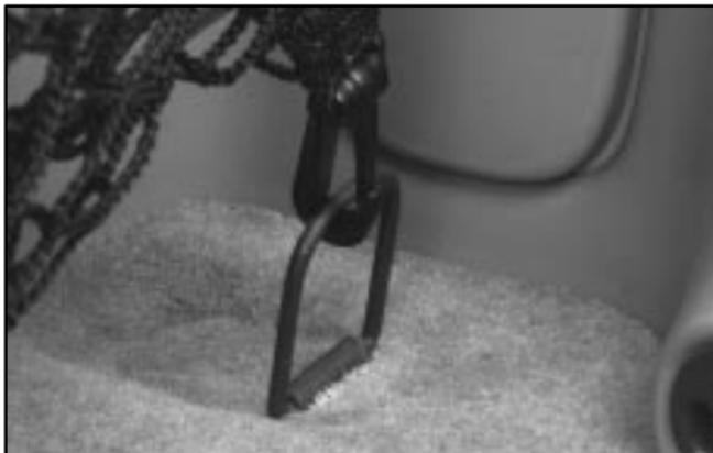
2. Attach the lower hooks to the metal rings on the floor.
