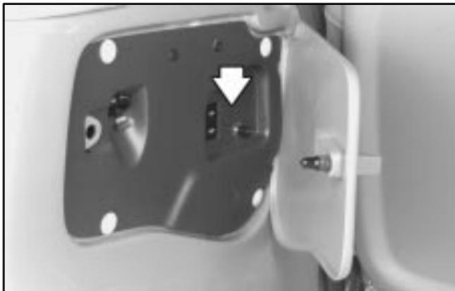
The switch and outlet for the air inflator system are located in the rear compartment on the driver's side next to the accessory power outlet.
