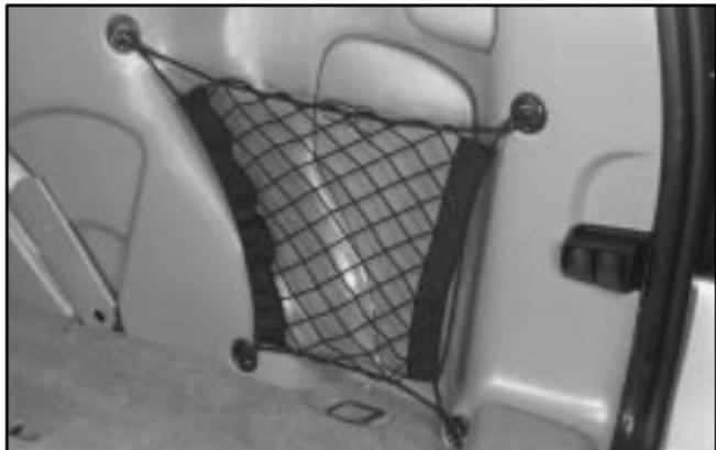
Attach the loops to the posts on the rear side panels, near the jack storage area.
