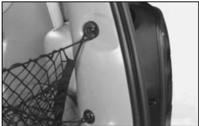
1. Attach the upper loops to the posts on either side of the liftgate opening (the label on the net should be in the upper left corner).
