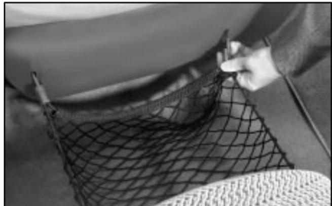
There is a storage net that stretches between the front seats. Pull the hooks toward the passenger's seat and insert them into the holes.
