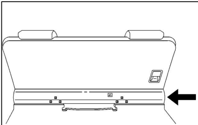
4. Put the tray sill, located on the back of the convenience center, to the upright position.
