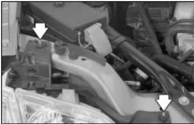
3. Remove the two wing nuts located on top of the headlamp assembly.
