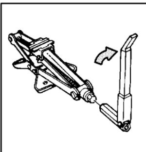
3. Attach the folding wrench to the jack, and turn the wrench clockwise to raise the jack head a few inches.
