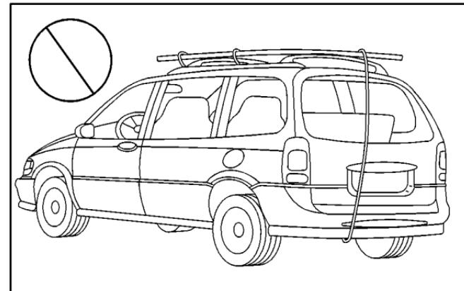
If you have the optional luggage carrier, you can load things on top of your vehicle. The luggage carrier has slats and side rails attached to the roof, as well as sliding crossrails and places to use for tying things down. These let you load some things on top of your vehicle, as long as they are not wider or longer than the luggage carrier.
