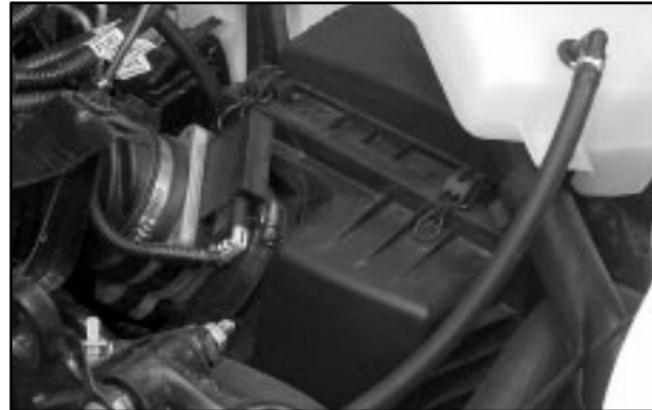
The engine air cleaner/filter is located at the front of the engine compartment, on the driver's side of the vehicle, under the engine coolant reservoir. See "Engine Compartment Overview" in the Index for more information on location.
