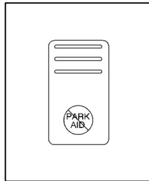
The rear PARK AID switch is located in the overhead console switchbank.
