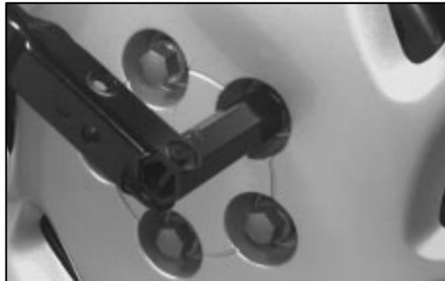
If your vehicle has the plastic “bolt-on” wheel covers, loosen them completely using the folding wrench, and remove the wheel cover.
