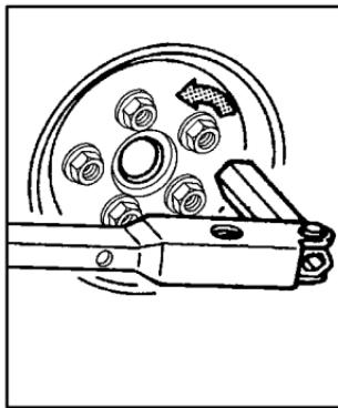
1. Loosen the wheel nuts -- but do not remove them -- using the folding wrench.
