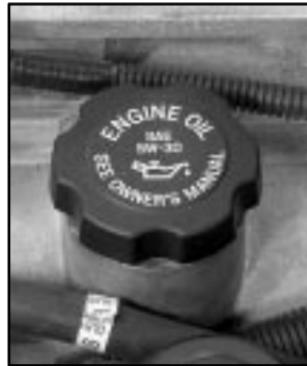
The engine oil fill cap is located behind the engine oil dipstick. See "Engine Compartment Overview" in the Index for more information on location.
