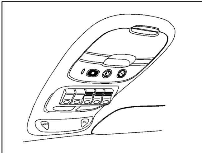
The optional front overhead console has reading lamps, a switchbank, storage compartments, OnStar® System buttons, an optional Driver Information Center (DIC) and optional HomeLink® Transmitter buttons. For information on the features listed see each of them in the Index.
