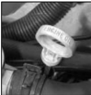
The engine oil dipstick is located at the front of the engine compartment, near the center. The dipstick handle has a bright, yellow loop design for easy identification. See “Engine Compartment Overview” in the Index for more information on location.
