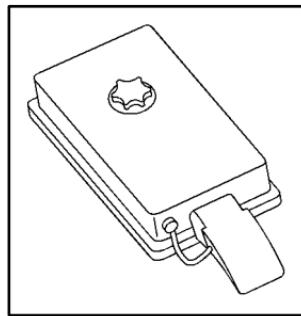
This fuse block is located in the engine compartment, in front of the windshield washer fluid reservoir. See "Engine Compartment Overview" in the Index for more information on location.
