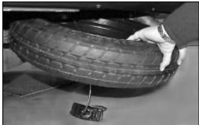
5. Grasp the compact spare tire with both hands and pull it out from under the vehicle.
