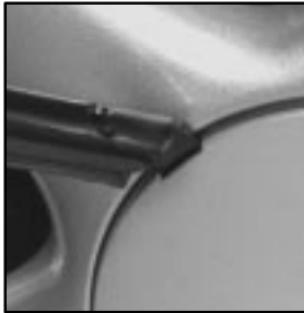
If your vehicle has aluminum wheels, use the handle of the folding wrench to pry the large center cap off.
