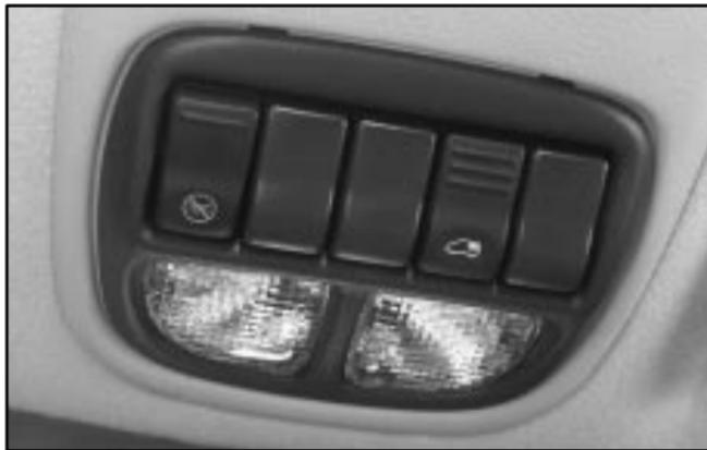
There are two reading lamps in the overhead console.
