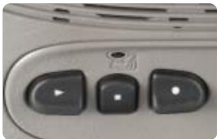
The Travel Note Recorder includes three buttons located in the overhead console.
