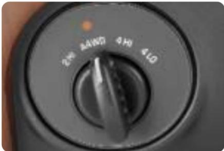
Envoy's four-wheel drive system rotary controls are located on the instrument panel.
