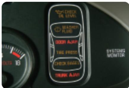
On equipped vehicles, the Systems Monitor buttons are located on the control panel to the right of the instrument cluster.
