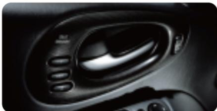
Your vehicle may be equipped with a two-driver memory function that is used to program and recall settings for the driver's seat and outside mirror positions. (The Driver Information Center (DIC) can also be programmed to personalize additional functions. See the DIC section of this booklet for more details.)
