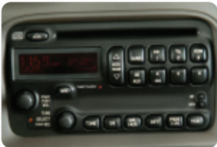
**Setting the clock:** Press and hold HR or MIN for two seconds. Then press and hold the HR button until the correct hour appears (AM or PM also appears). Adjust minutes by pressing and holding the MN button. To set time to an FM station's Radio Data System setting, press and hold both HR and MN until UPDATED and the clock symbol appear on the display. If the time is not available from the station, NO UPDATE appears in the display.
