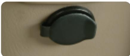
Your vehicle is equipped with an accessory power outlet that can power a variety of accessories.
