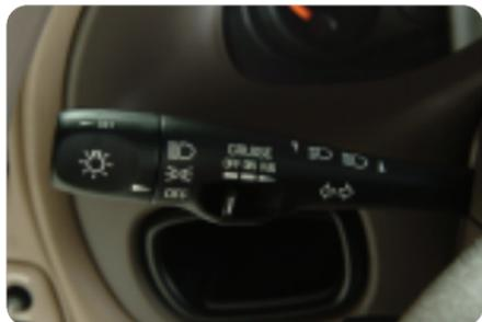
Use Cruise Control for steady driving on relatively straight, uncrowded roads. The controls are located on the Turn Signal/Multifunction Lever on the left side of the steering column.
