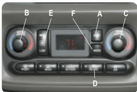
**Automatic Operation:** Press the AUTO button (see “A” above) for automatic control of inside temperature, air delivery mode and fan speed.
