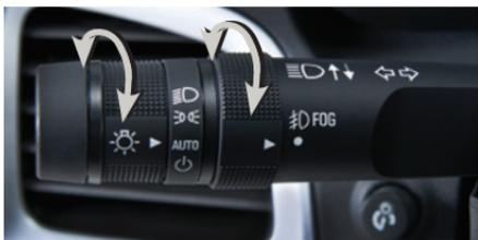
**TIP:** Push the lever to turn on the high beam headlamps; pull the lever to return to low beam operation. Pull the lever to activate the flash-to-pass feature.
