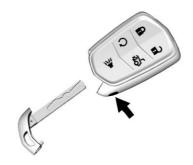
Press the key release button near the bottom of the transmitter to remove the key. The key can be used for the driver door.
