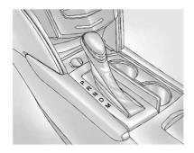
P : This position locks the wheels. It is the best position to use when starting the engine because the vehicle cannot move easily.
