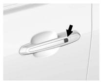
If equipped, use the Keyless Access system to lock and unlock the door. When the doors are locked and the RKE transmitter is within 1 m (3 ft) of the driver door handle, press the lock/unlock button. When unlocking from the driver door, the first press unlocks that door; press again within five seconds to unlock all passenger doors. See Remote Keyless Entry (RKE) System Operation ⇒ 28.
