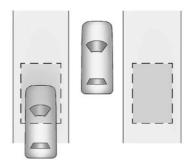
The SBZA sensor covers a zone of approximately one lane over from both sides of the vehicle, or 3.5 m (11 ft). The height of the zone is approximately between 0.5 m (1.5 ft)
