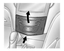
If equipped with storage behind the climate control system, touch the bottom of the climate control system panel to open. There is a USB port inside. See the infotainment manual.
