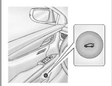
To open the trunk, press from inside the vehicle or press twice quickly on the Remote Keyless Entry (RKE) transmitter, or press the touch pad on the rear of the trunk above the license plate after unlocking all doors. See Remote Keyless Entry (RKE) System Operation ⇒ 40 and Trunk ⇒ 40.
