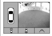
If equipped, a view of the area in front of the vehicle displays in the center stack. The view displays after shifting from R (Reverse) to a forward gear, or by pressing CAMERA in the center stack, and when the vehicle is moving forward slower than 8 km/h (5 mph). If equipped, the front view camera also displays when the Front Parking Assist system detects an object within 30 cm (12 in).
