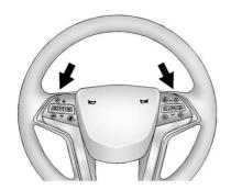
Tap Shift allows the driver to manually control the automatic transmission. To use Tap Shift, the shift lever must be in M (Manual Mode). If equipped, the controls are on the back of the steering wheel. Tap the left control to downshift, and the right control to upshift. A Driver Information Center (DIC) message indicates the gear the vehicle is in. See Manual Mode ♀ 195.
