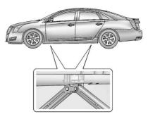
Position the jack lift head at the jack location nearest the flat tire, as shown. The jack must not be used in any other position.
