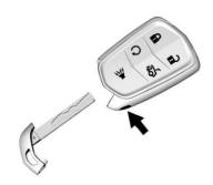
There is a key inside the Remote Keyless Entry (RKE) transmitter that is used for locking/unlocking the driver door and for locking the rear seatbacks so they cannot be folded. See Rear Seats  $\Rightarrow$  62.
