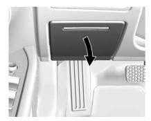
The instrument panel fuse block is in the instrument panel, on the driver side of the vehicle. To access the fuses, open the fuse panel door by pulling down at the top. Press in on the sides of the door to release it from the instrument panel.
