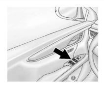
The power windows work with the ignition in ACC/ACCESSORY or ON/RUN/START, or when Retained Accessory Power (RAP) is active. See Retained Accessory Power (RAP) ⇒ 190.
