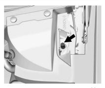
The vehicle has a remote negative (-) ground location. It is located on the driver side of the engine compartment. See Engine Compartment Overview
