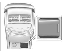
An indicator light on the outlet turns on to show it is in use. The light comes on when the ignition is in ON/RUN, equipment requiring less than 150 watts is plugged into the outlet, and no system fault is detected.
