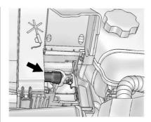
The vehicle has a remote positive (+) terminal under a trim cover. It is under the battery cover on the driver side of the engine compartment. See Engine Compartment Overview ⇒ 240. Always use this remote positive terminal
