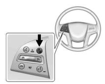
The Collision Alert control is on the steering wheel. Press to set the FCA timing to Far, Medium, or Near, or on some vehicles, Off. The first
