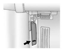
Pull the hood release lever with this symbol on it. It is inside the vehicle on the lower side of the instrument panel.
