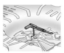
Turn the wrench counterclockwise to remove the fastener rod.
