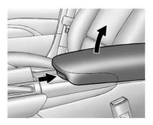
Press the button and lift to access the storage area. There is a power outlet, auxiliary jack and USB port(s) inside. See Power Outlets \$\Display 110\$ and the infotainment manual.
