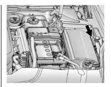
The electrical cord is on the driver side of the engine compartment, between the fender and the engine compartment fuse block.
