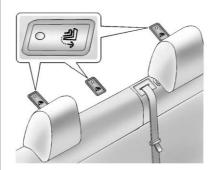
The top tether anchors are under the covers, behind the rear seat, on the filler panel. Be sure to use an anchor
