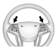
Tap Shift allows the driver to manually control the automatic transmission. To use Tap Shift, the shift lever must be in M (Manual Mode). Vehicles with this feature have indicators on the steering wheel. The controls are on the back of the steering wheel. Tap the left control to downshift, and the right control to upshift. A Driver Information Center (DIC) message indicates the gear the vehicle is in.
