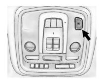
On vehicles with a rear window sunshade, the sunshade switch is on the overhead console. The sunshade only operates with the ignition in ON/RUN/START.
