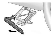
Raise the vehicle by turning the jack handle clockwise. Raise the vehicle far enough off the ground so there is enough room for the road tire to clear the ground.
