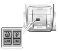
If equipped, the sunroof operates when the ignition is on or in ACC/ACCESSORY, or when Retained Accessory Power (RAP) is active. See Retained Accessory Power (RAP) \$ 277.
