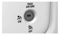
If the vehicle does not have an airbag on-off switch, it may have a passenger sensing system. See Passenger Sensing System ⇒ 81.
