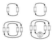
Use this rotation pattern when rotating the tires if the vehicle has polished forged aluminum dual rear wheels. The spare wheel can be used in any position in the event of a flat tire, and can be rotated with the rear inner wheels. After the flat tire is repaired, if the spare is not on one of the inner rear positions, it
