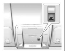
If equipped, the power sliding rear window works when the ignition has been turned to ACC/ACCESSORY or ON/RUN, or when Retained Accessory Power (RAP) is active. See Retained Accessory Power (RAP) ⇒ 277.
