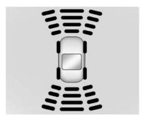
The instrument cluster may have a parking assist display with bars that show "distance to object" and object location information for the Parking Assist system. As the object gets closer, more bars light up and the bars change color from yellow to amber to red.
