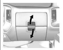
To access the upper glove box, unlock with the key and pull up on the handle.
