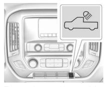
The cargo lamp provides more light in the cargo area or on the sides of the vehicle, if needed. The lights inside the pickup box and/or on the outside mirrors also turn on, if equipped.
