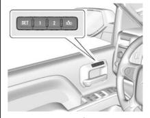
The SET, 1, 2, and (Exit) buttons on the driver door are used to manually store and recall memory settings for the driver seat, outside mirrors, and adjustable pedals.
