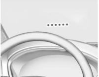
When your vehicle approaches another detected vehicle too rapidly, the red FCA display will flash on the windshield. Also, eight rapid high-pitched beeps will sound from the front, or both sides of the Safety Alert Seat will pulse five times. When this Collision Alert occurs, the
