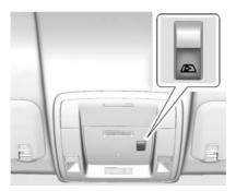
If equipped, the power sliding rear window works when the ignition has been turned to ACC/ACCESSORY or ON/RUN, or when Retained Accessory Power (RAP) is active. See Retained Accessory Power (RAP) ⇒ 277.
