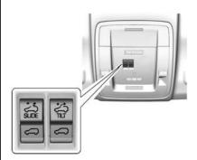
If equipped, the sunroof operates when the ignition is on or in ACC/ ACCESSORY, or when Retained Accessory Power (RAP) is active. See *Retained Accessory Power* (RAP) ⇒ 277.
