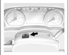
\(\textcal{\textcal{\textcal{\textcal{L}}}}\): Press this button to make the front and rear turn signal lamps flash on and off. Press again to turn the flashers off.
