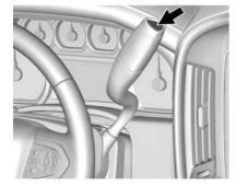
Vehicles with an automatic transmission have a Tow/Haul Mode. The Tow/Haul Mode adjusts the transmission shift pattern to reduce shift cycling. This provides
