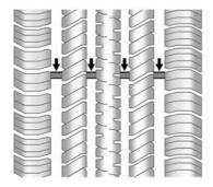
Treadwear indicators are one way to tell when it is time for new tires. Treadwear indicators appear when the tires have only 1.6 mm (1/16 in) or less of tread remaining. Some
