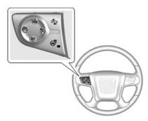
The FCA control is on the steering wheel. Press to set the FCA timing to Far, Medium, Near, or Off.
